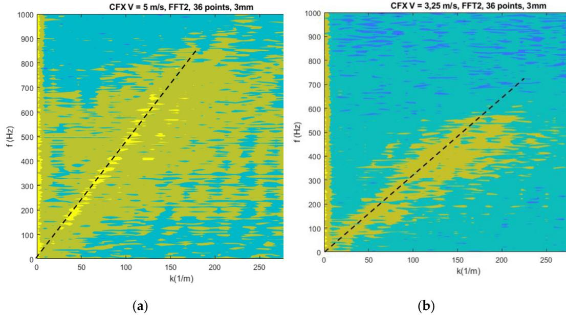
**Fig. 2.** Frequency-wavenumber spectrum determining the phase velocity of movement of turbulent vortexes.
