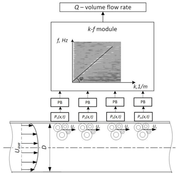
Fig. 4. Pre-processing block on the functional scheme of a clamp-on sonar flow meter.
