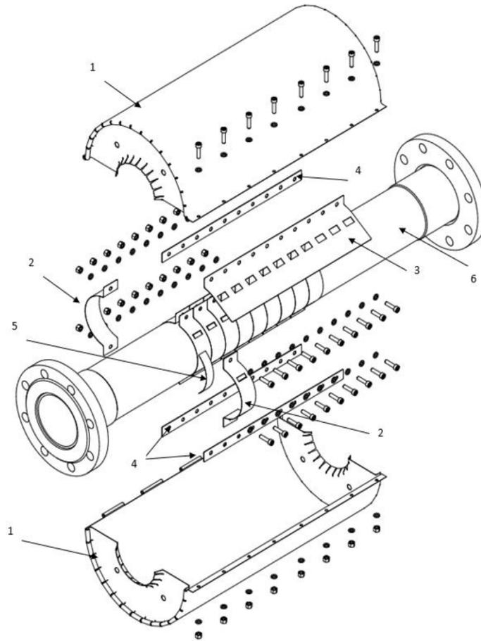
Fig. 3. Mechanical part of clamp-on flow meter.
