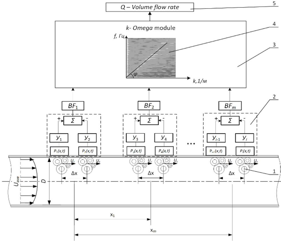
Fig. 1. Functional structure of the non-invasive flow measurement method.
