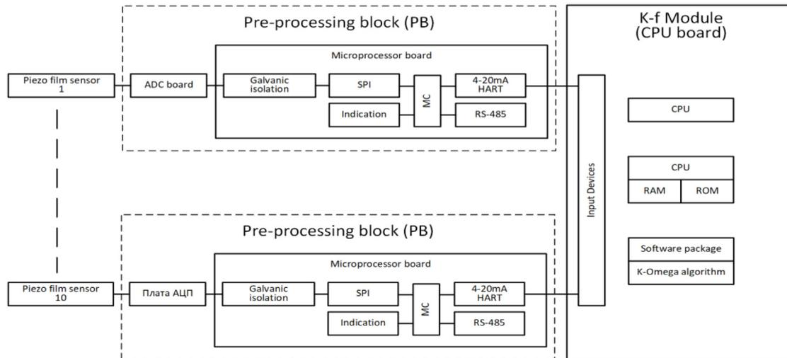
**Fig. 5.** Functional structure of the clump-on sonar flow meter “K-Omega P1”.
