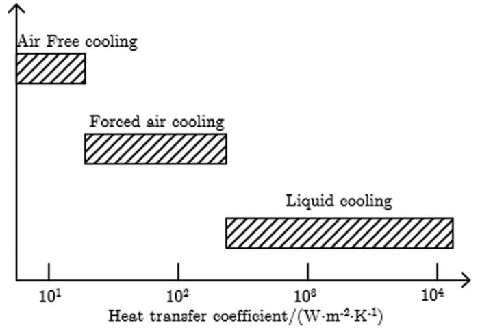
**Fig. 2.** Comparison of heat transfer coefficients of different cooling methods [16].
