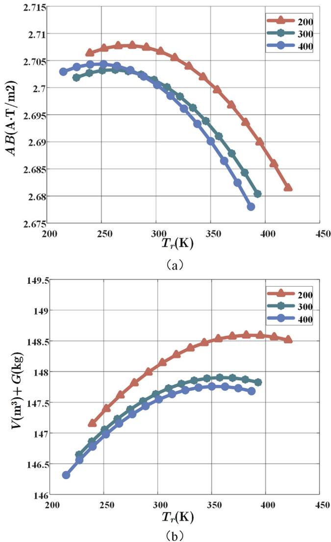
**Fig. 4.** Comparison of Pareto frontier curves under different population numbers: (a) electromagnetic size and temperature rise and (b) volume + weight and temperature rise.
