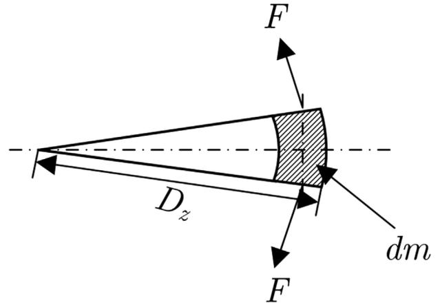
Fig. 1. Force analysis of micro mass units of the rotor.
