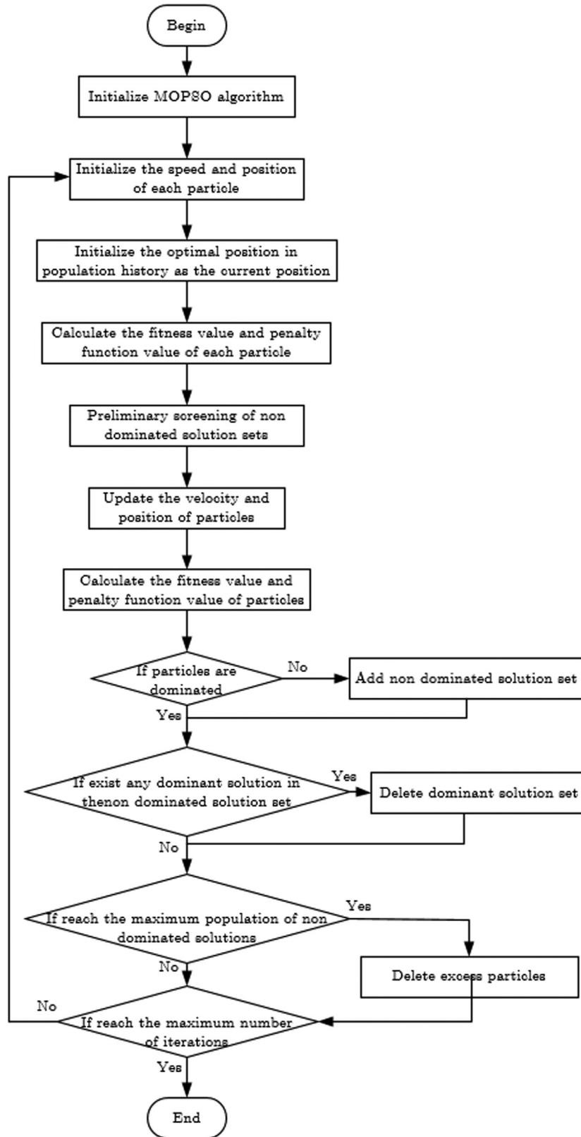
Fig. 3. Flowchart of MOPSO algorithm.
