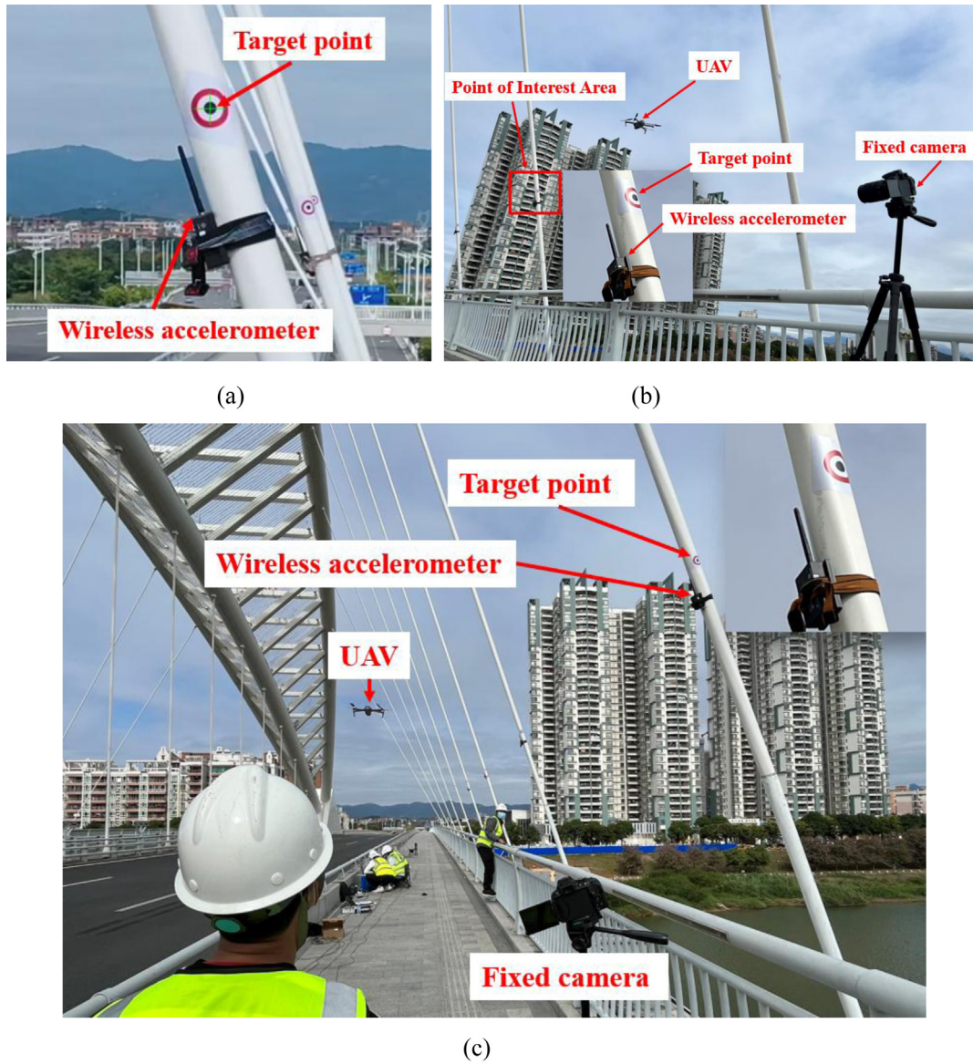
Fig. 18. (a) Target point and accelerometer; (b) and (c) Measurement layout of Conghua Bridge.
