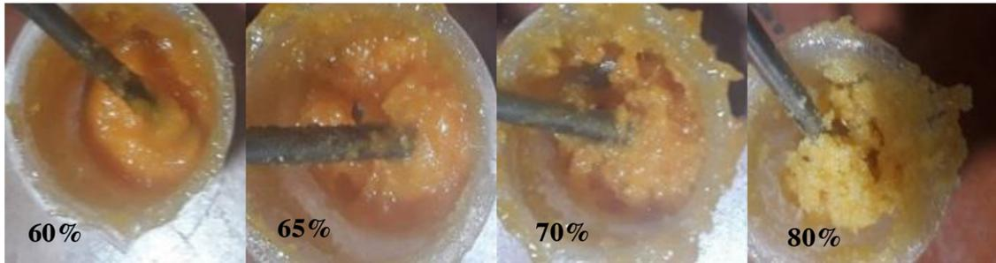
**Fig. 5.** Slurry composition with different solid loading (NaCl) percentage.
