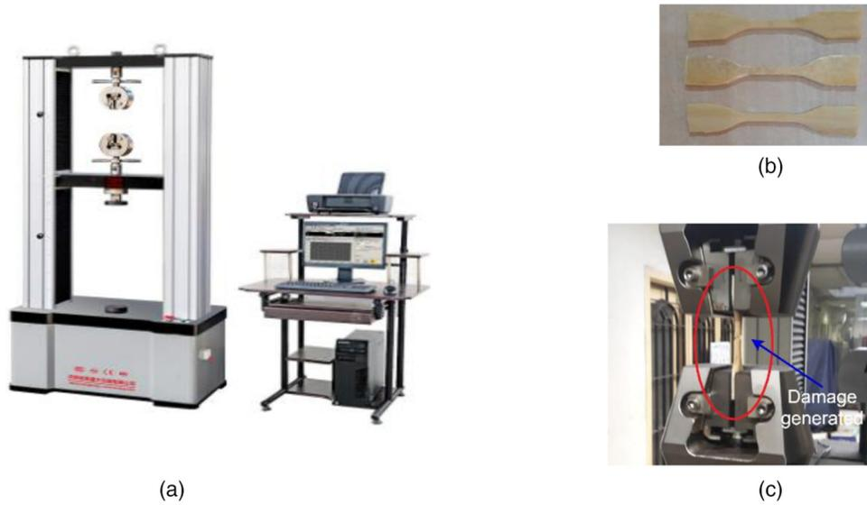
**Fig. 4.** Tensile strength testing. (a) WDW-100 computer control electronic universal testing machine; (b) tensile strength specimen (ASTMD 412-C); (c) Fracture generation during the test.
