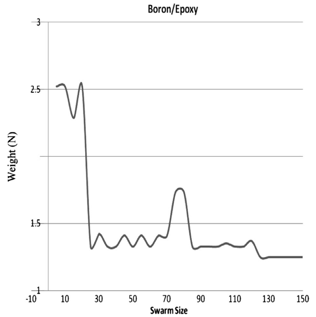
Figure 9. Variations of weight of Boron/Epoxy drive shafts with swarm size.
