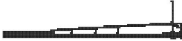
Figure 13: Final topology design with ERPM ( C=509.829J )
