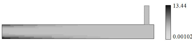
Figure 10: Distribution of the element strain energy with void OCM elements ( C=2296.64J )
