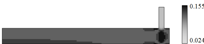
Figure 9: Distribution of the original element strain energy ( C=195.04J )
