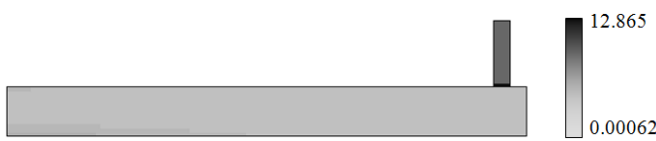
Figure 11: Distribution of the strain energy with moderate OCM elements ( C=1238.36J )
