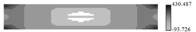
Figure 28: Sensitivity values associated with the topology generated by the 3 rd iteration ( f_1=64.17 Hz)
