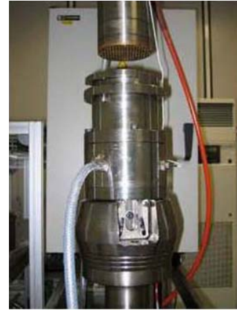
Fig 8: Experimental setup for compression test
