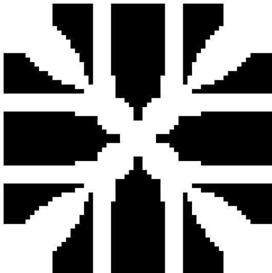
Fig. 3. Optimal distribution of high conductive material based on BESO method.
