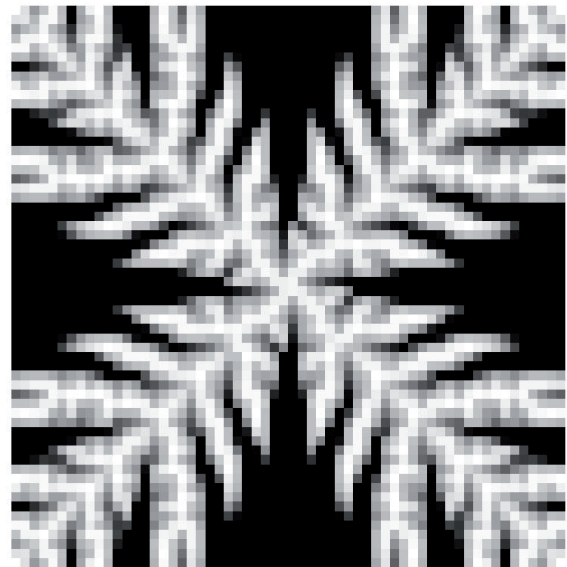
Fig. 5. Optimal distribution of high conductive material based on SIMP method.
