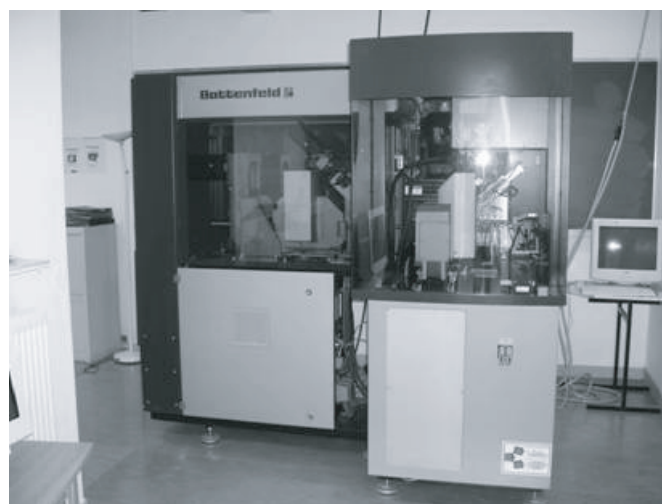
Fig. 1. Two-colours Battenfeld microsystem 50.
